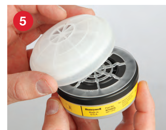
Place the pad filter support on top of the cartridge, "groove side up". Then, snap the filter cover onto the cartridge or N750037 filter holder and cover (if a cartridge is not being used).
