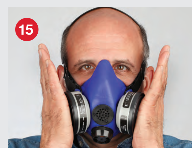
Negative Pressure Seal Check: Place the palm of each hand over the two cartridges or filters so they are completely sealed and inhale. Hold your breath for 5 seconds. If you have a good seal, the facepiece will be pulled inward toward your face.
